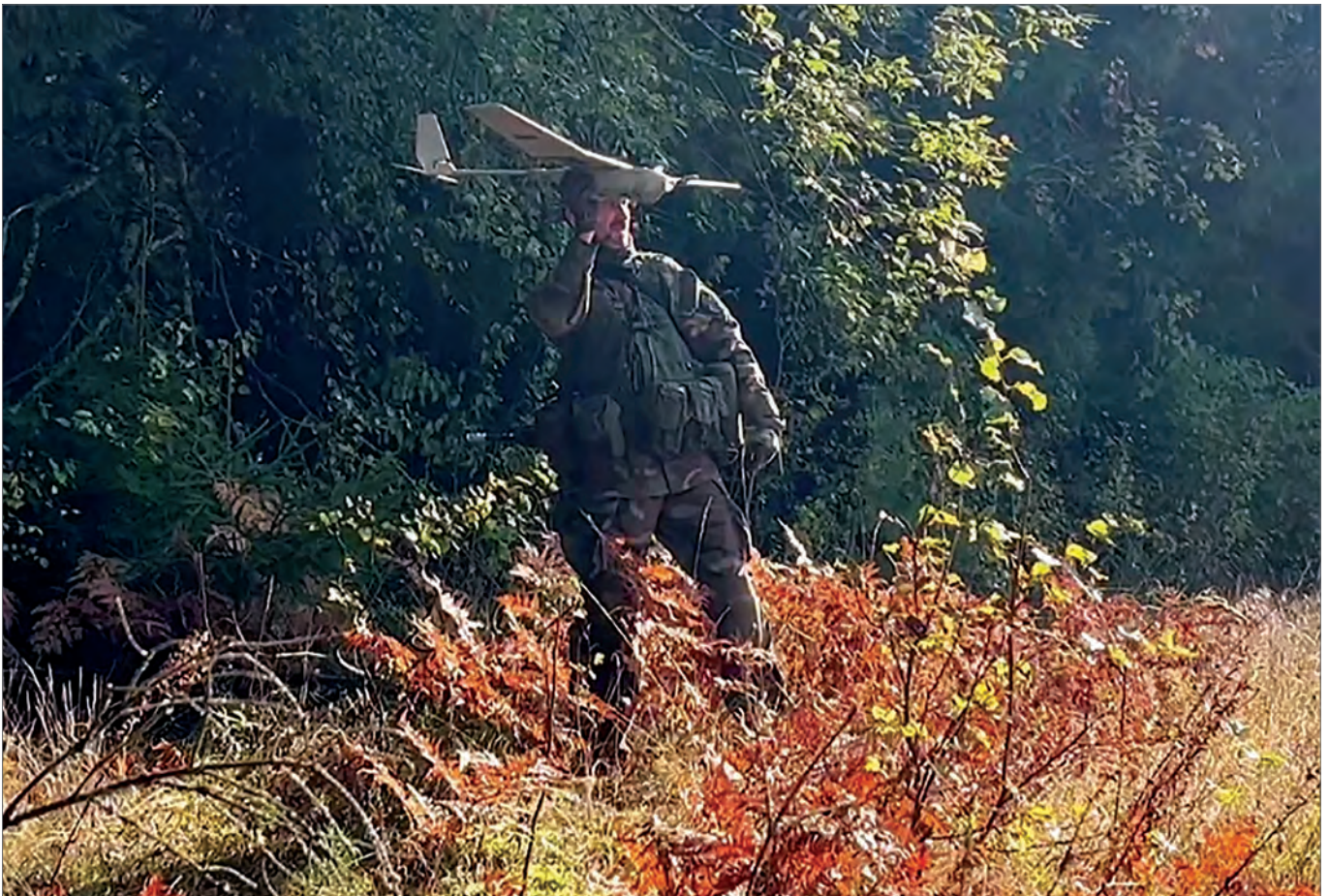
Granta Autonomy's Hornet-XR hand-launched UAS can perform autonomous missions even in "radio silence" (Photo: Granta Autonomy)
