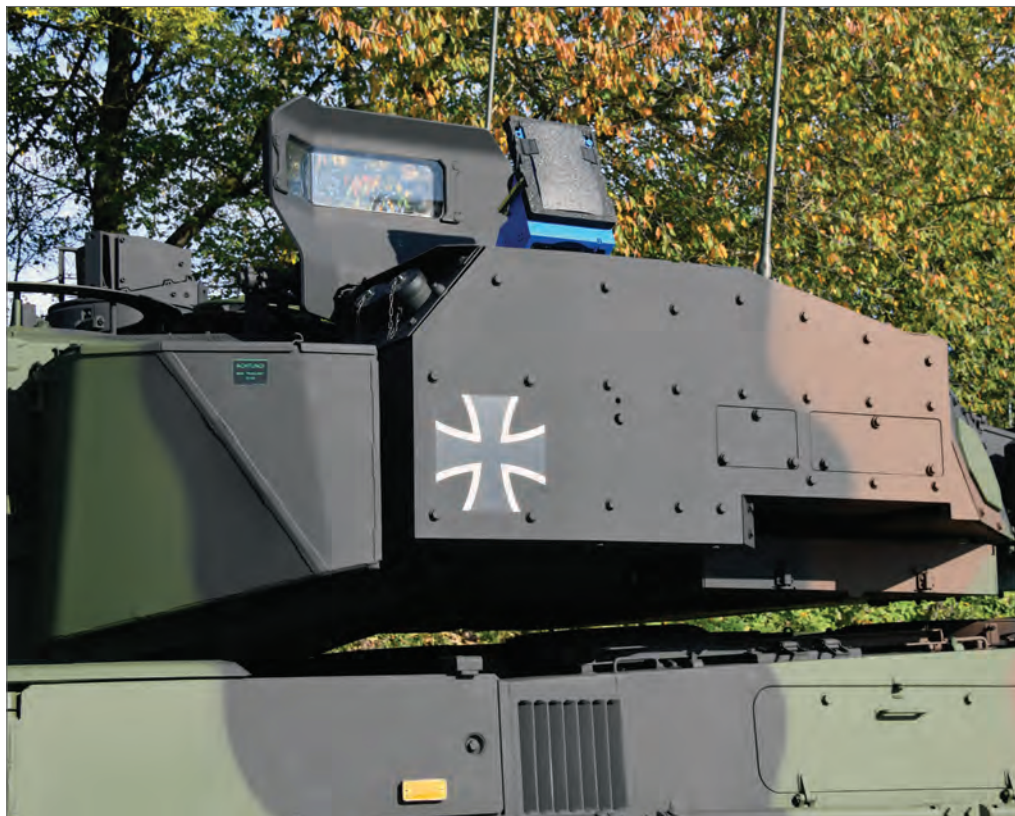
The Trophy launcher on the left side of the turret. Note the two new launchers of the 76 mm smoke discharger system integrated in the Trophy launcher box (Photo: Ralph Zwilling)
