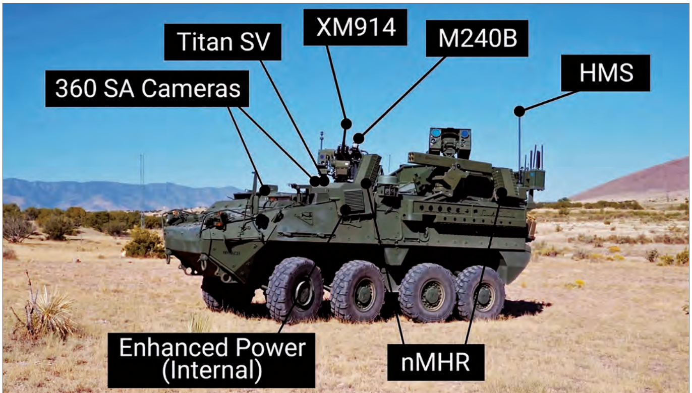
The kinetic and non-kinetic weapons on the DE C-UAS Stryker include the guns, Titan jammer, 360-degree situational cameras, AESA next-generation radars, and laser weapon system (Photo: Screenshot)
